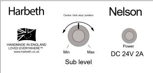
The Nelson connector plate features a sub level control that allows you to adjust the bass (up and down) to suit your music taste and preferences. Please remember that each Nelson is independent, requiring its own separate setup.
