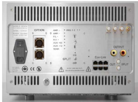
Rear view: A lock secures access to the rail system and the inside of the enclosure.
