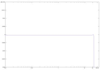
The Naim DSP filter response and passband ripple, input sample rate 48kHz
