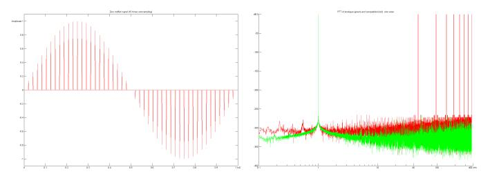
The same 1kHz signal as before (left) and its spectrum (right), sampled originally at 48kHz but now zero-stuffed with 15 zero-valued samples between each adjacent pair of original samples. The sample rate is now (16 x 48 =) 768kHz
