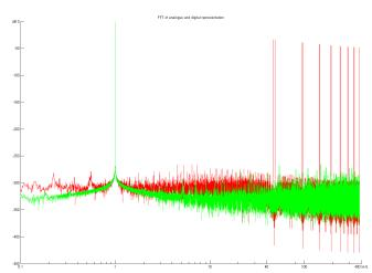
Spectral analysis of the original signal (green trace) and the unprocessed DAC output (red trace).
