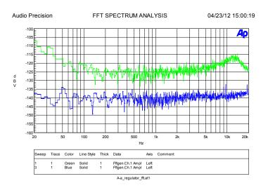
Wideband noise spectra, 20Hz-20kHz, of the outgoing HiCap (green trace) and the latest HiCap fitted with the Naim Discrete Regulator (blue trace). The midband improvement is about 15dB  $(5.6 \times)$  with still larger improvements at low and high frequency
