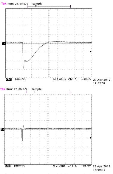
Transient performance comparison of the old regulator circuit (top graph) and Naim Discrete Regulator (bottom graph), showing the change in output voltage when a load current of 0.65A is suddenly applied (rise time 250ns). The much faster settling time of the Naim Discrete Regulator is obvious
