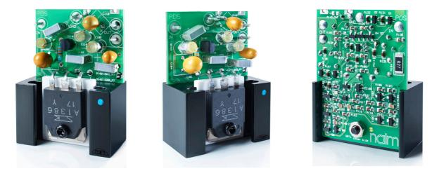
A regulator circuit of almost this form was first used in the NAP 500 power supply, since when the concept has been further refined by incorporating an enhanced voltage reference. This topology, which was benchmarked against various alternatives and refined over the two year period, has proven itself to be inherently low noise and capable of fast recovery to transient current demands. It also has the advantage that it works equally well for both positive and negative supply rails.
