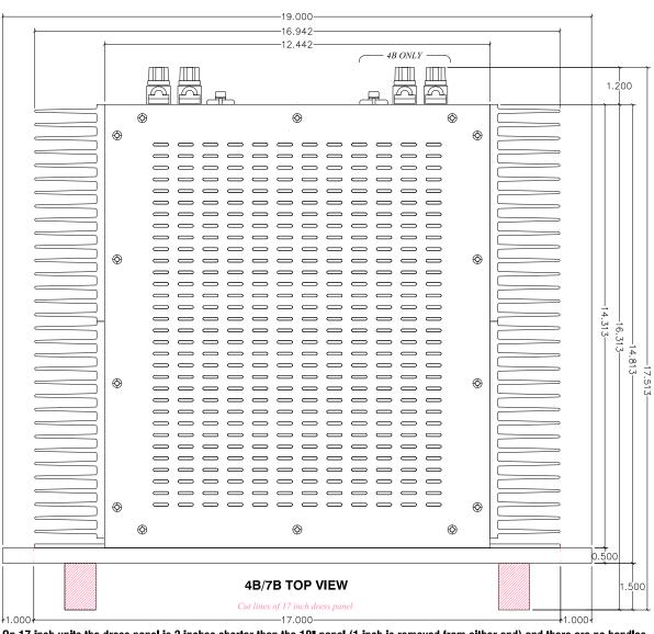
On 17 inch units the dress panel is 2 inches shorter than the 19" panel (1 inch is removed from either end) and there are no handles.
